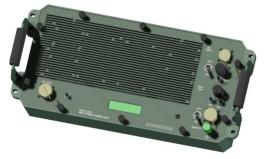
The RCPU can charge all types and ratings of Nickel Cadmium and sealed and vented lead acid batteries. It can also drive system load of up to 150W simultaneously. RCPU comes with three variants of output DC voltages: 12V, 24V, 48V.
