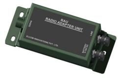
RAU can be easily connected to the Radio set using a radio interconnect cable. On the other end, spring loaded binding posts are provided for connecting single pair of field wire to a remote located telephone. DC power for RAU operation is derived from either Radio set or an external battery. ELCOM's Advanced Field Telephone (AFT1001), can be connected to single pair of wire and operated in radio mode.
